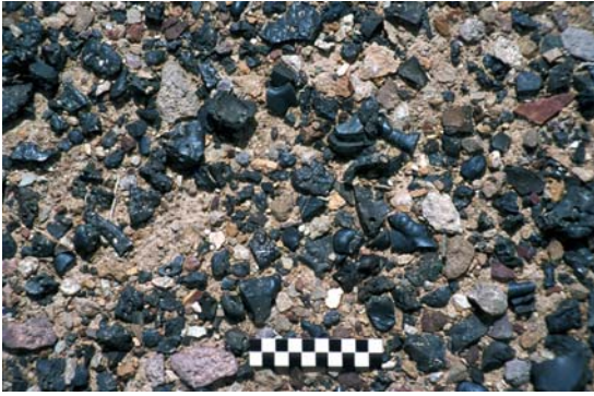
Metallurgy in Arabia. Fig. 3 Batin in Wadi Nam near Ibra has the oldest slag. As is typical for the third millennium, the slag had to be crushed to expose and collect the copper drops and prills (scale 10 cm).
